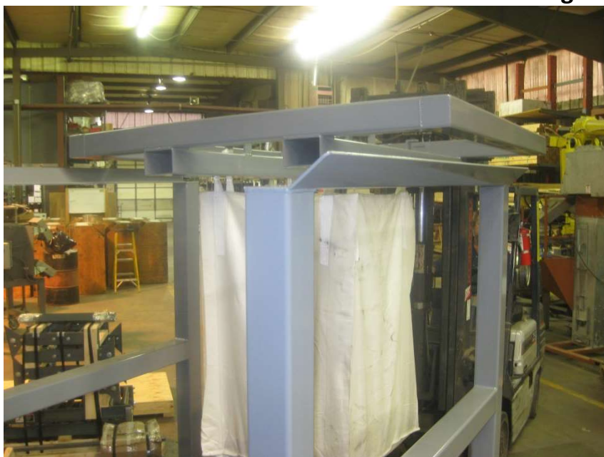
SPIDER ASSEMBLY being moved via Fork Truck into CRADLE
