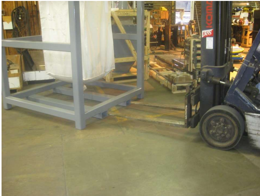
CRADLE holding Super Sack (in the Spider Assembly) being moved to place on top of Hopper
