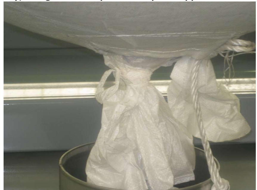
CRADLE holding Super Sack (in the Spider Assembly) being moved to place on top of Hopper
