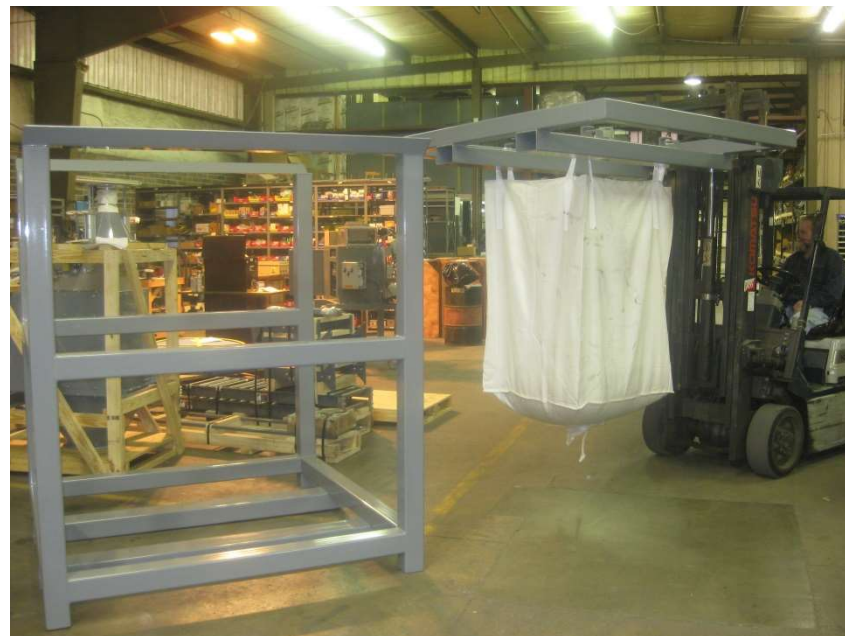
SPIDER ASSEMBLY being moved via Fork Truck into CRADLE
