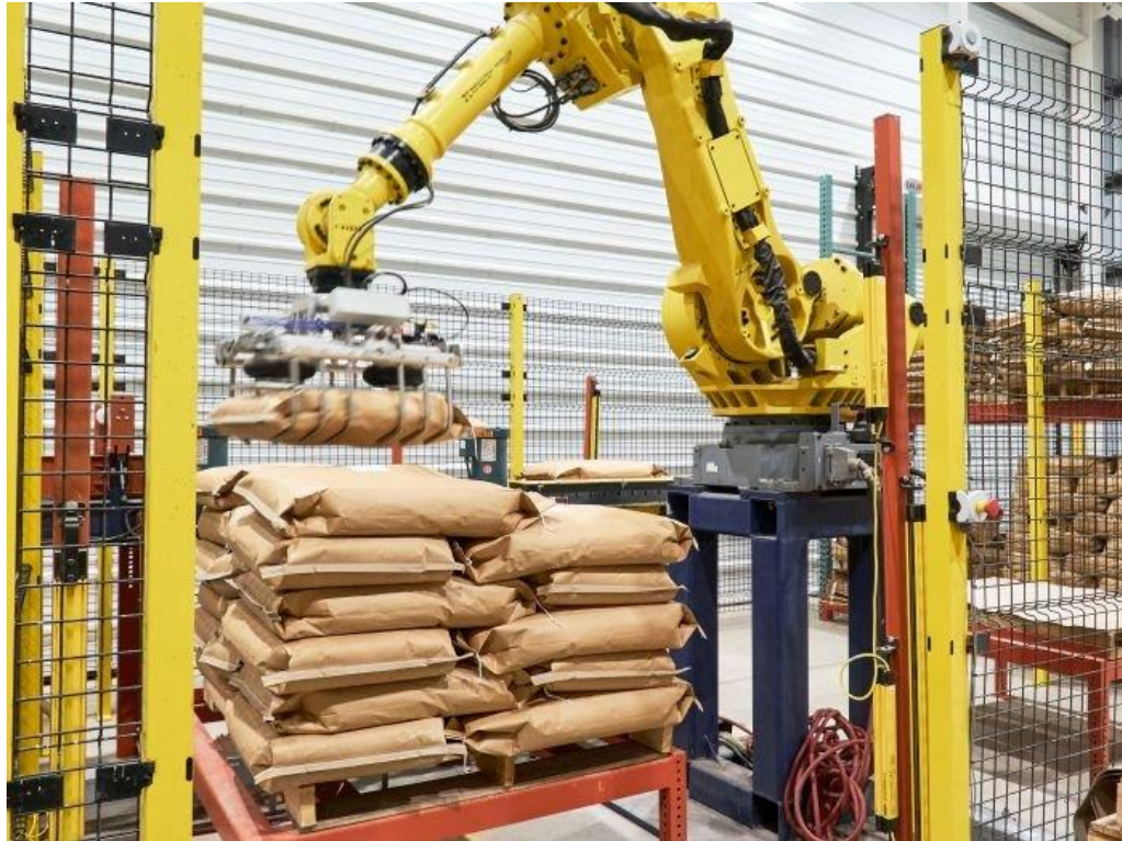
A JEM International robot stacks bags of feed on pallets at the Feed Technology Center. (Ann Reus)
